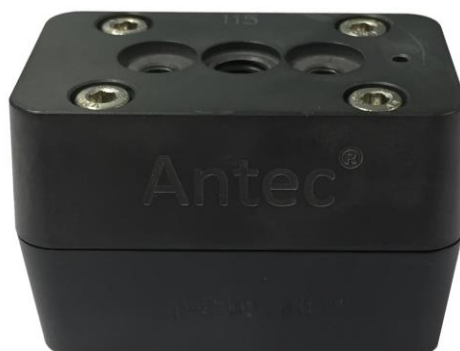
Figure 14. \mu -PrepCell inlet and WE block fixed with 4x M4 stainless steel allen screws.
