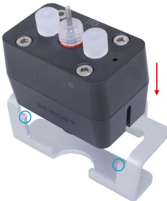
Figure 8. Inserting the \mu -PrepCell 2.0 into the cell holder. The groove in the sides of the cell should slide through the plane with the notches. The cell will snap into place (locked by the notches).
