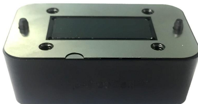
Figure 11. PEEK WE block with MD working electrode and stainless steel spacers.
