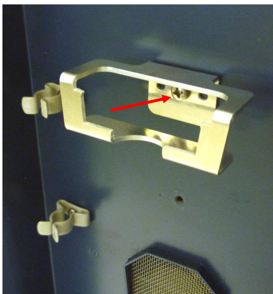
Figure 7. \mu -PrepCell holder mounted on the centre position in the ROXY potentiostat oven compartment.
