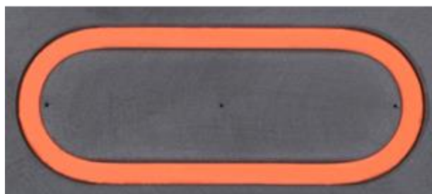
Figure 21. Active area (AUX) of the \mu -PrepCell 2.0 inlet block with Silicone O-ring.
